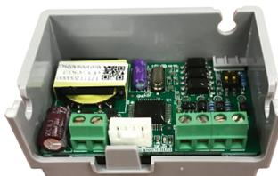
The 24V Interface for Carrier VRF systems is a device that enables the use of a conventional 24VAC thermostat with indoor units. The Interface receives 24VAC signals for cool, heat and fan. This translates these commands to the system's communication protocol and sends the commands to the indoor units over the HA/HB communication bus.
