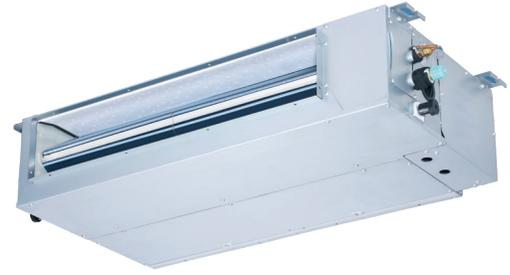
The Carrier VRF Low Static Ducted (Slim Profile) Unit is only 8-1/4" in height, making it an ideal candidate for narrow soffit space applications. Air return can be rear or bottom, but rear is default.
