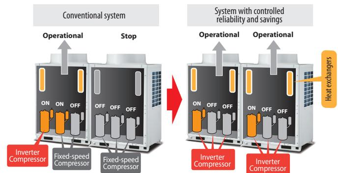
Using greater heat exchanger volume is more efficient
