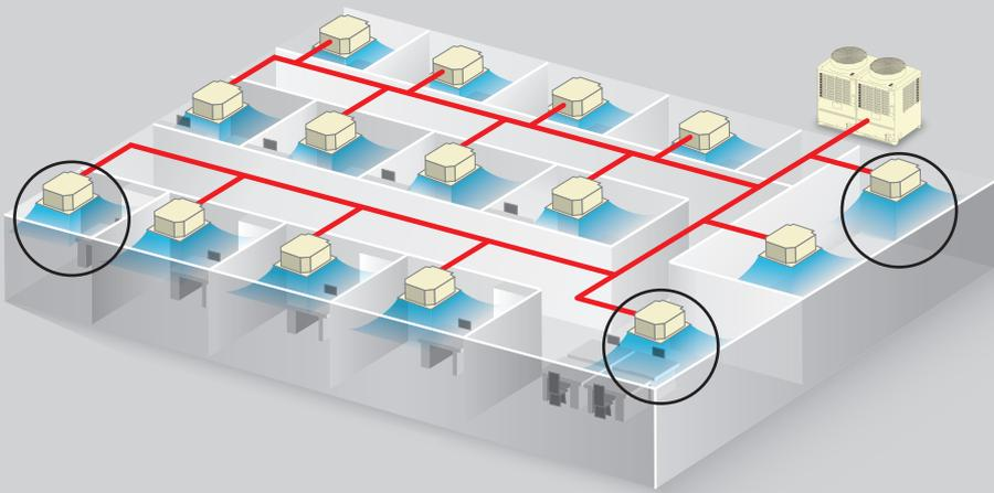
Refrigerant flow is adjusted to maintain consistent individual temperature control
