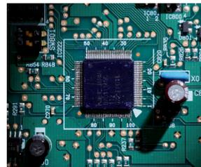
The vector-controlled inverter quickly converts current into a smooth sine curve to achieve smoother operation of the compressor's DC motor.
