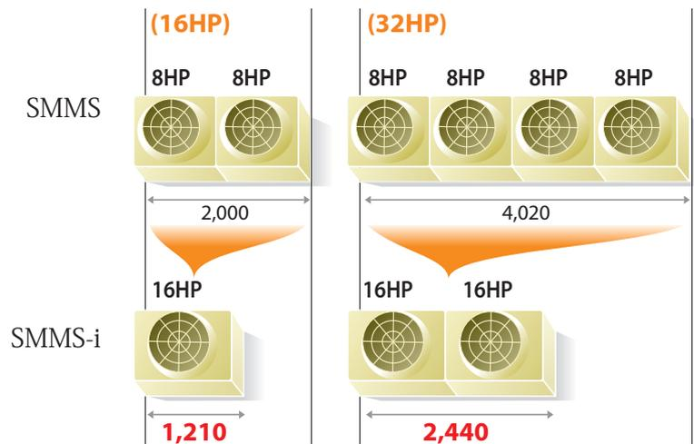
A 16HP system installation now occupies only 2/3 the footprint and weight of two units previously required.
