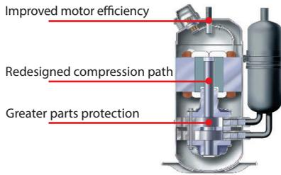
Optimization of discharge port positioning and blade thickness reduces the compression loss and friction resistance. Increasing the surface area of the rotor magnets and the addition of slits realize greater efficiency and reduced noise.
