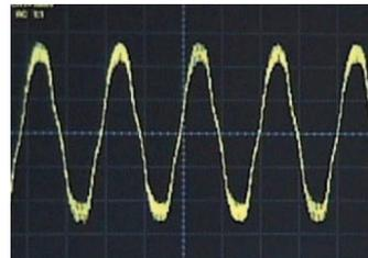
The fast-calculating vector-controlled inverter produces a smooth sine curve that improves operating efficiency.
